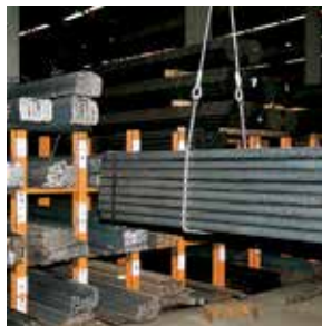
Combined rope/chain suspension gear for particularly rough use
