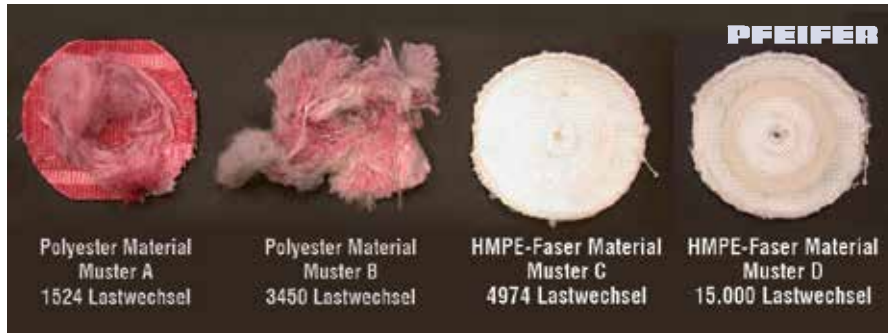
The abrasion of HMPE fibres compared to polyester
